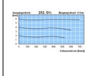
ToolReg Regulator with relieving function, outlet pressure 4 bar, supply pressure max. 25 bar, female/male thread G 1/4, aluminium
