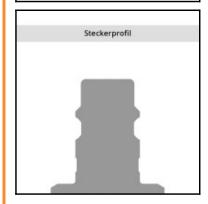
Quick coupling straight-through, hose barb 13mm (1/2), nominal diameter 7,8, <35 bar, brass nickel plated, seal NBR  $\,$
