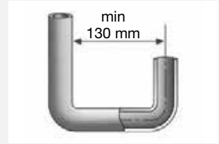
● Minimum clearance of U-shape bends
