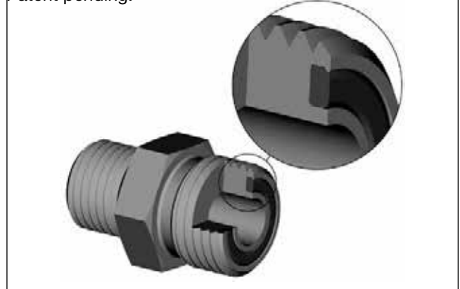
Fig 2 – Captive O-ring Groove (CORG) cutaway
