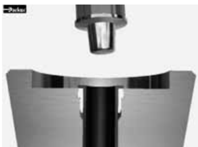
As soon as the defined flange contour is achieved, the orbital movement stops and the pin withdraws
