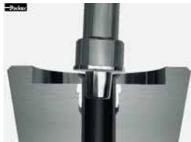
As soon as the flat working surface of the pin contacts the tube end, the flanging process begins
