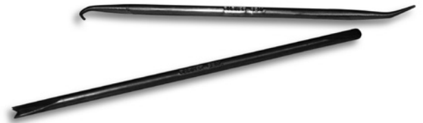
Fig. 5.10 O-ring assembly aids
