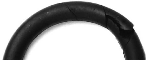
Fig. 10.10 Twisted O-ring with cuts in surface
