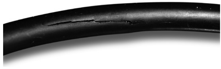
Fig. 10.11 O-ring damaged by explosive decompression
