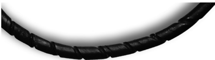
Fig. 10.9 Twisted O-ring with spiral markings
