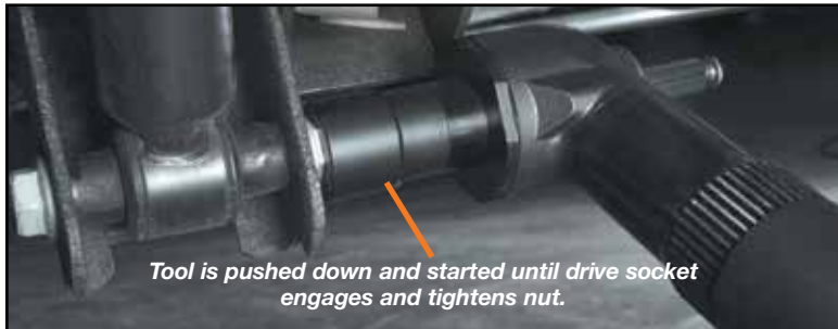
Hold socket fits over bolt and prevents it from rotating.
