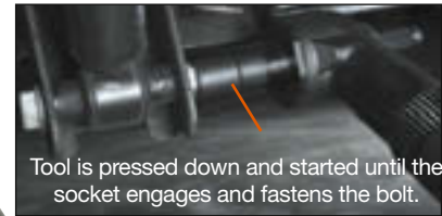
Holding socket fits over the bolt and prevents it rotating.
